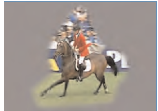
Figure 2. Helios uses Ph.C motion estimation to identify and track the “area of interest” within the content. It then dynamically reframes the image and processes the background to concentrate the energy of the compression encoder onto that area of interest.
